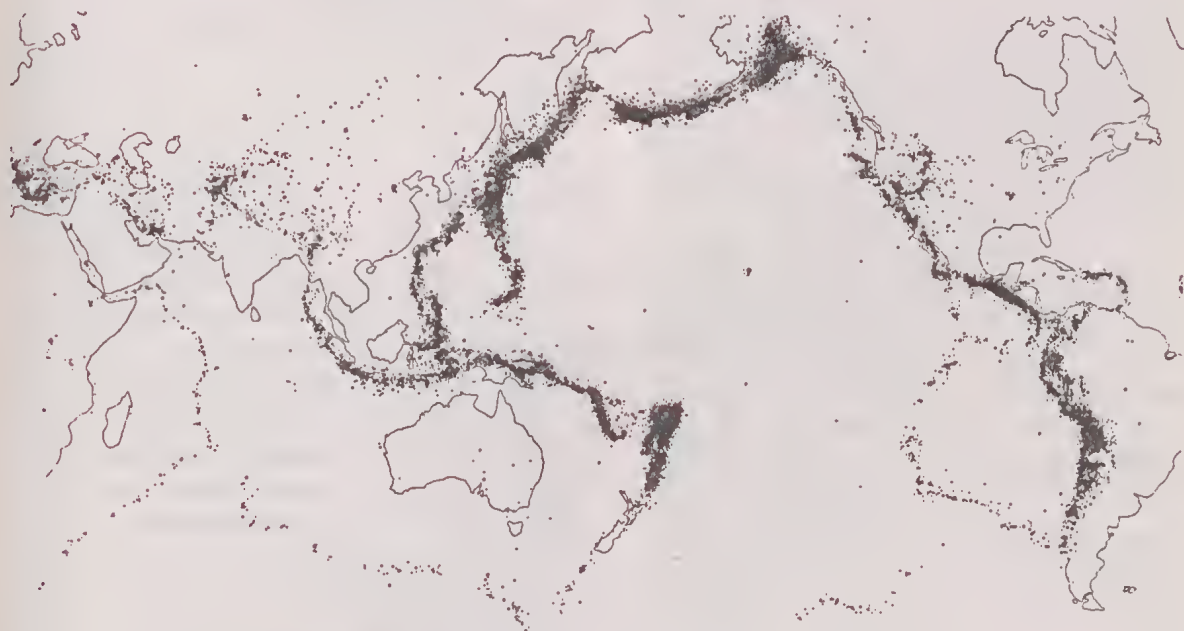
FIG. 5b—Dots represent the epicentres of earthquakes with focal depths greater than 100 km. After Barazangi and Dorman 1968. Their association with tectonic plate borders is very marked. Australia's position well within the Indo-Australian plate accounts for its relative freedom from such earthquakes.
